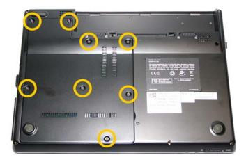
**4.** Using a flat edge tool, preferably plastic, insert its tip in the depressed area as shown in Figure 6 and carefully lift up the cover to remove.
